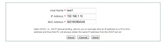
Figure 4-20 Static DHCP Settings\_Example A
