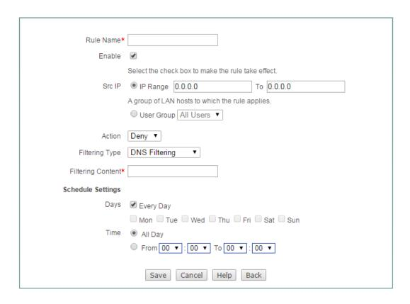
Figure 9-7 Access Control Rule Settings DNS Filtering
