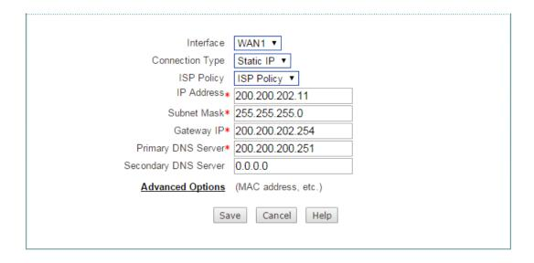
Figure 4-3 Static IP Connection Setup
