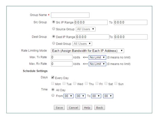
Figure 8-2 Fixed Rate Limiting Setup
