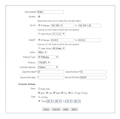
Figure 9-8 Access Control \_Example 1\_step 1
