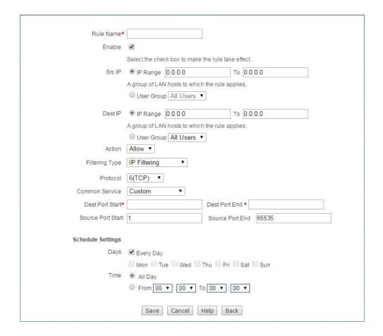
Figure 9-4 Access Control Rule Settings\_IP Filtering
