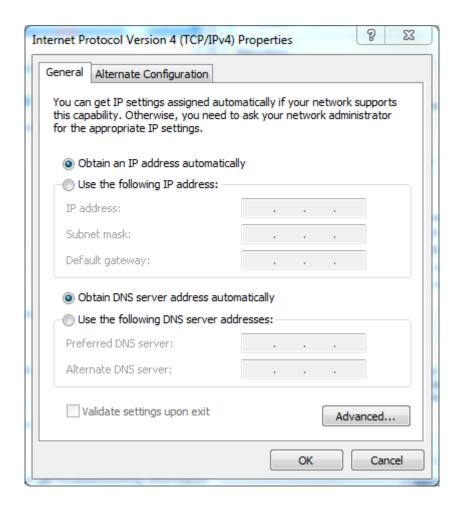
Figure Appendix- 2 Automatically Configuring TCP/IP with DHCP
