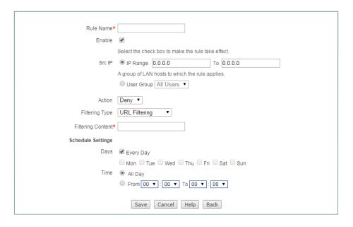
Figure 9-5 Access Control Rule Settings\_URL Filtering
