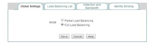
Figure 4-8 Full Load Balacing
