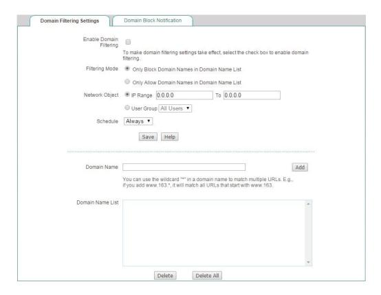
Figure 9-13 Domain Filtering Settings
