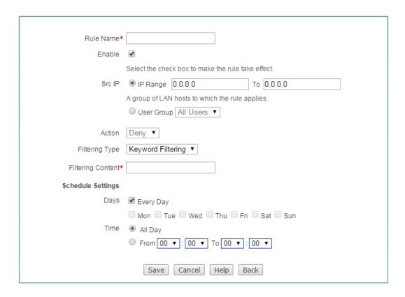
Figure 9-6 Access Control Rule Settings\_Keyword Filtering
