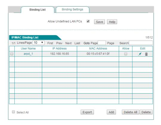
Figure 6-5 IP/MAC Binding List - Example Two
