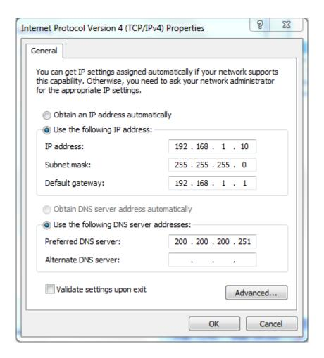
Figure Appendix- 1 Manually configuring TCP/IP
