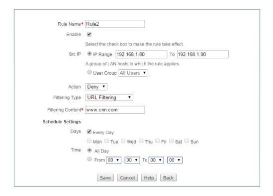
Figure 9-12 Access Control \_Example 2\_step 2
