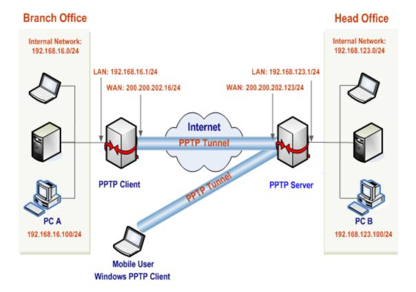
Figure 10-34 Network Topology - the Device Acts as a PPTP Server
