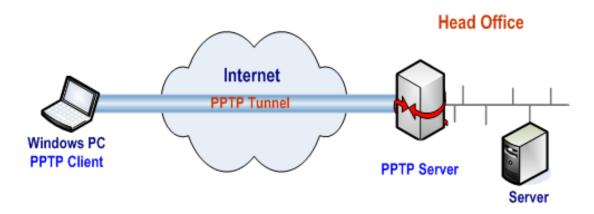
Figure 10-1 Typical Application of PPTP
