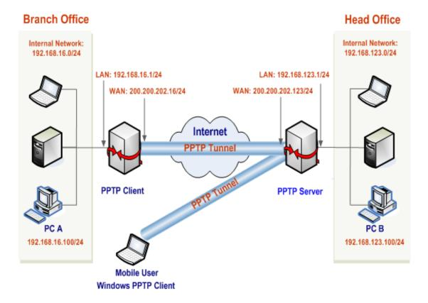
Figure 10-25 Network Topology - the Device Acts as a PPTP Server
