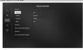
Depending on the settings made at the separate 'Zone Setup' menu under the 'Setup Menu' section discussion, the applicable Zone can be configured and managed via this 'Zone Controls' window.
