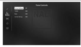
The T 777 has three Tone Control levels – Treble, Bass and Center Dialog. Bass and Treble controls only affect the low bass and high treble leaving the critical midrange frequencies free of coloration. The Center Dialog ('Dialog' in the VFD) control boosts the 'presence' of the midrange region improving intelligibility of speech.
