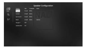
Every surround-sound system requires "bass-management" to direct low-frequency content from any or all channels to the speakers best able to reproduce it. For this function to operate correctly, it is important that you correctly identify your speakers' capabilities. We use the terms "Small" and "Large" (and "Off") but note that physical size may be irrelevant.
