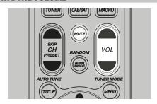
In addition to the Volume knob, use the HTR 8's [VOL riangle / riangle riangle ] to adjust the "master volume" of the T 777 raising or lowering the channels altogether. A momentary keypress will change the master volume by 1 dB increments. If you hold down [VOL riangle / riangle ], the master-volume change will "run-on" until the key is released.
