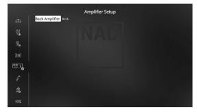
If the surround back speakers are not used in the main zone, their surround back amplifier channels could be assigned for Back, Front (Bi-Amp), Height 1, Height 2, Zone 2, Zone 3 and Zone 4.
