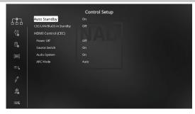
The T 777 supports HDMI Control (CEC) and Audio Return Channel (ARC) functions. Both functions are possible if external devices that also support both features are interconnected with the T 777 via HDMI connection.
