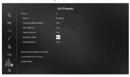
While at "Save Current Setup to Preset" menu line, use [▶] to save the settings above to "Preset 2". When you recall "Preset 2" using the remote control (for HTR 8, "A/V PSET" + "2"), the above preset values allocated at "Preset 2" (preset settings as shown in the OSD captures at Step 4) will be recalled and effected at the current source.
