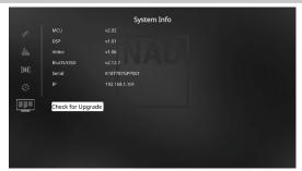
"System Info" displays information about current firmware versions of MCU, DSP, Video and BluOS/ OSD as well the unit's serial number and IP address. The System Information shown above is for reference only.
