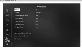
The T 777's simple but powerfully flexible system of "A/V Presets" allows you to customize virtually every aspect of your audio-video playback, and recall them with a single key-press. The parameters "DSP Options" and "Tone Controls" accessible via the "Main Menu" together with "Listening Mode Setup", "Speaker Setup" and "Display Setup" configurable through "Setup Menu" are stored together as a single A/V Preset.
