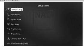
The Setup Menu allows one to customize the operation of the T 777 to the ancillary equipment used in one's specific AV system. Unless your system exactly matches the factory defaults as shown in the accompanying Quick Start Guide, you will need to use the setup menu to configure the inputs of the T777.
