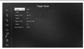
The T 777 features three configurable +12V DC Trigger Output that can be used to activate a component or system it is fed into. A Trigger Input is also available to turn on the applicable link it is associated to.
