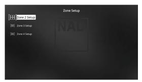
The Zone feature allows one to simultaneously experience in different zones of the house multiple sound sources from all enabled Sources as well as from Front Input and Media Player.
