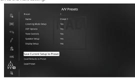
While at "Save Current Setup to Preset" menu line, use [ $\$ ] to save the above settings to Preset 1. Below OSD will be shown, affirming that the above settings are now saved to "Preset 1".
