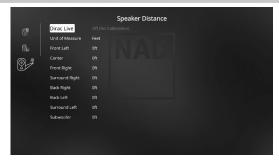
Your system's speaker distance settings are a subtle but important refinement of your setup. Informing the T 777 of the loudspeaker-to-listener dimensions of each speaker automatically imposes the correct delays, optimizing imaging, intelligibility and surround-sound ambience. Enter your dimensions with precision within about 1 foot (30 cm).
