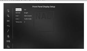
The Vacuum Fluorescent Display (VFD) and On-Screen Display (OSD) can be shown in various ways by navigating through the parameters at the 'Display Setup' menu.
