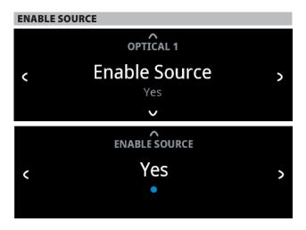
One can enable/disable a Source via this option. This is particularly useful if only few Sources are used thereby bypassing unused sources.
