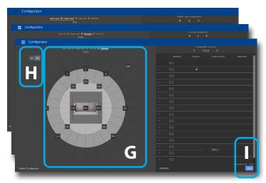
Configuration is shown. A four digits description is given following this order:, "Base Layer. LFE. Height Layer. Top Layer".
