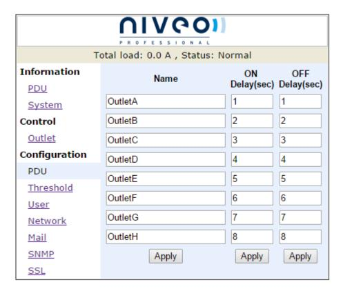
Note: After PDU is plugged into main power, PDU system will start to sequentially turn on the output socket according to the pre-set delay time in PDU web interface. The factory default setting for delay time is one second for each outlet; therefore the 8 ports PDU will take 8 seconds, 24 ports PDU will take 24 seconds to complete start-up procedure.
