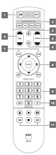
The SR 10 remote control handset handles the key functions of the C 389. It can also control up to 4 devices. SR 10 will operate up to a distance of 23ft (7m). Two AA batteries should be fitted in the battery compartment at the rear of the remote control handset. Ensure that the batteries are correctly oriented and installed as indicated on the base of the battery compartment.
