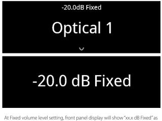
At Fixed volume level setting, front panel display will show "xx.x dB Fixed" as the volume control is adjusted.
