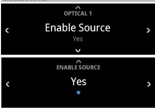
One can enable/disable a Source via this option. This is particularly useful if only few Sources are used thereby bypassing unused sources.
